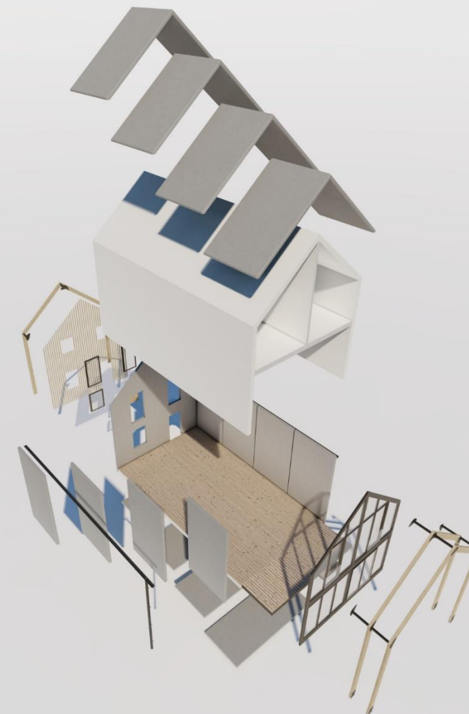
ConHouse house construction scheme
